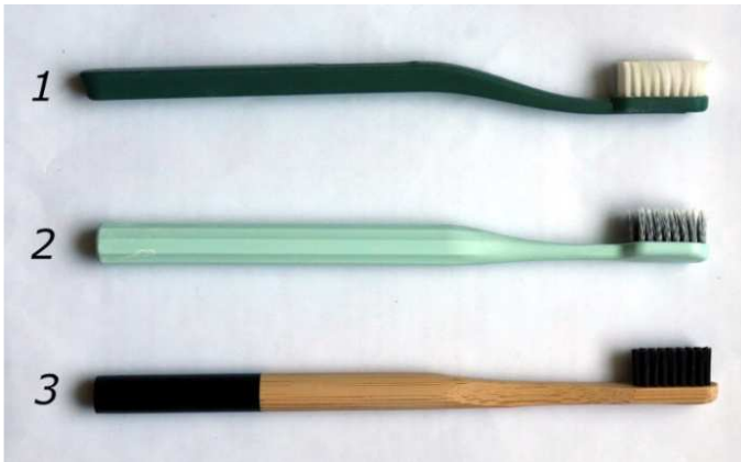
Fig. 2. Toothbrushes made of various materials. 1. Recycled plastic, 2. Polylactic acid (PLA), looks like plastic but is fully biodegradable, 3. Bamboo (handle) and biodegradable fibre (bristles).
